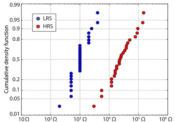
Fig. 6. Normal probability plot of LRS and HRS of 27 cells on the same chip.
